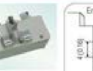
SMD TEST FIXTURE 9699 Direct connection type. For measuring SMDs with electrodes on the bottom, DC to 120 MHz, test sample dimensions: 1.0 mm (0.04 in) to 4.0 mm (0.16 in) wide, max. 1.5 mm (0.06 in) high
