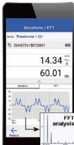
Waveform observation/FFT analysis
