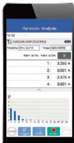
Check power quality by analyzing harmonics up to the 30th order
