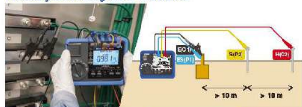
3-pole method using 4-terminal measurement Measure ground resistance values of several ohms or less
