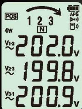
Positive phase sequence display
