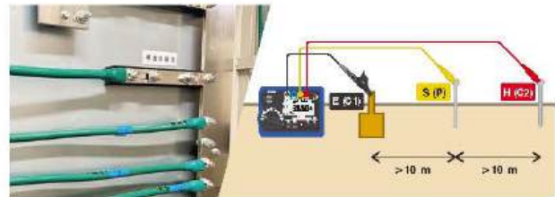
3-pole method Precisely measure ground resistance
