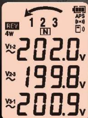
Negative phase sequence display
