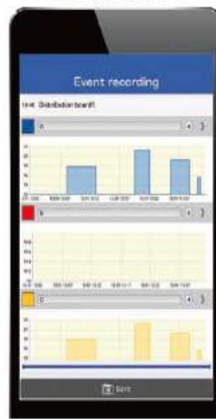
Record the occurrence of intermittent leakage current
