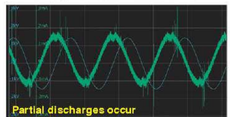
Current and voltage waveforms when 1.0 kV AC is applied to a stator with a pseudo-defect
