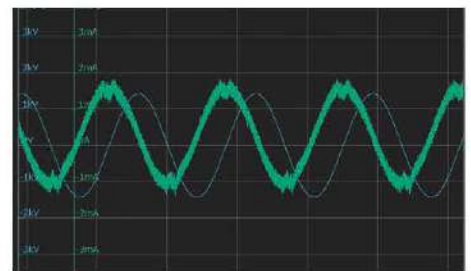
Current and voltage waveforms when 1.0 kV AC is applied to a non-defective stator
