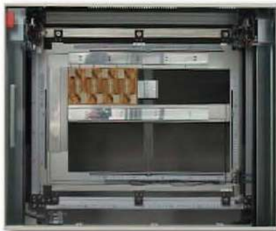
Fixing flexible boards with tension frames
